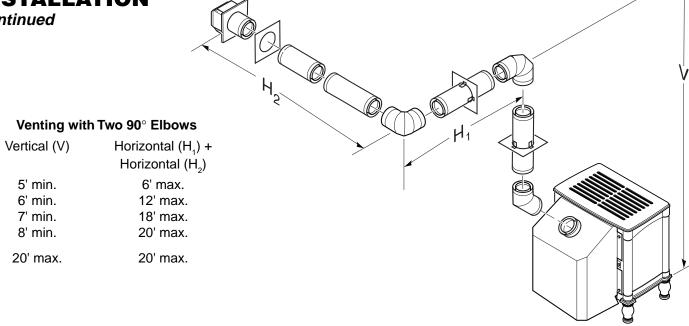
Figure 29 - Horizontal Termination Configuration for Rigid Venting Using Two 90° Elbows with Termination at 90° with Stove
